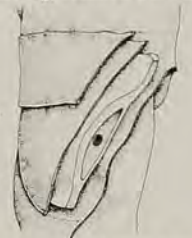
Cutaway view of knee pocket and pad
