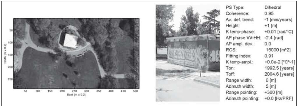
Figure 8 - Example of structure forming a dihedral. Left: aerial photo, center: ground photo, right: estimated parameters.
