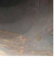
Fig11(right) Refractory condition after 40 fire cycles
