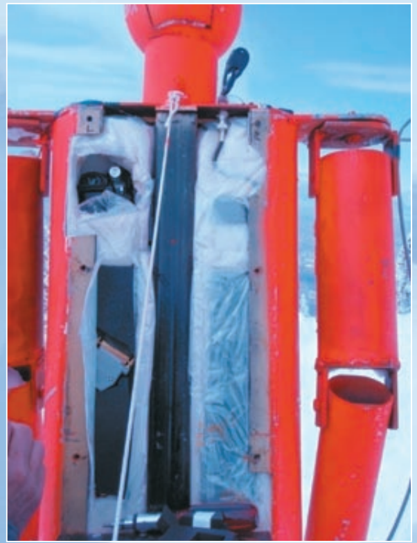
A closeup of Iron Man reveals camera and instrumentation used to collect acceleration data during the experiment. Both photos by Mike Jenkins
