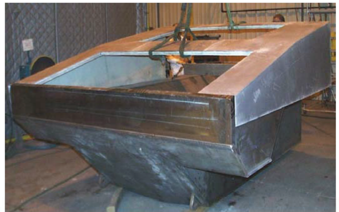
Figure 36. Prototype Future Combat Vehicle Titanium Hull Section
