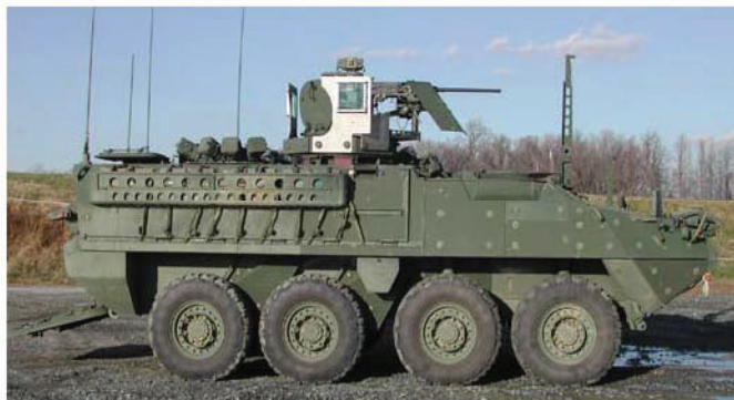
Figure 33. Titanium Gunners Overhead Protected Gun System on RV and RSV Stryker
