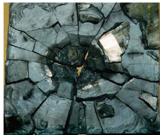
Figure 22 Functionally Graded Titanium Monoboride/Titanium Plate
