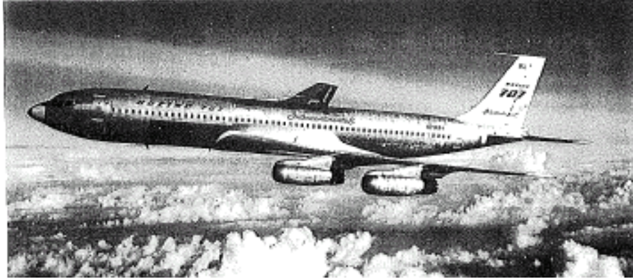
Figure 6. Boeing 707 Maiden Flight December 20, 1957, powered by 4 – P&W JT4s or Rolls-Royce Conway Turbojets. First Passenger Flight October 26, 1958 by Pan American World Airways
