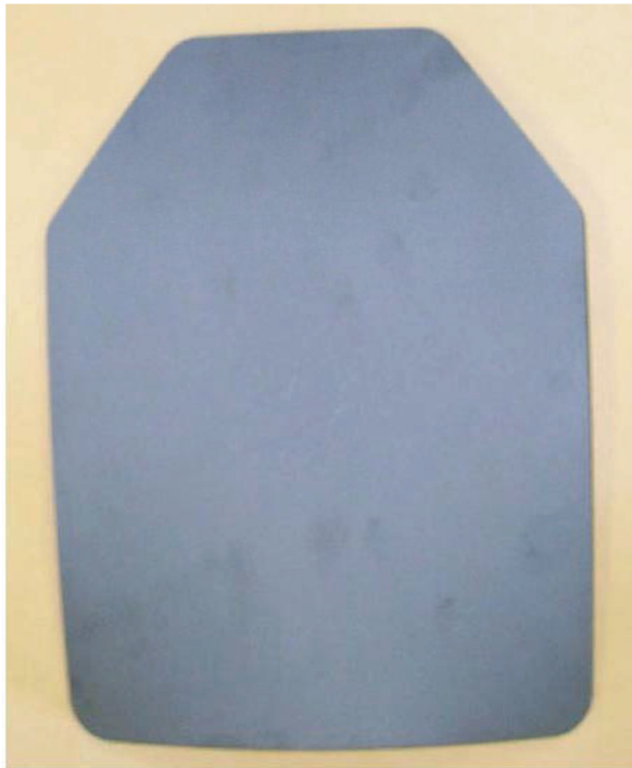
Figure 18. Hot-Pressed Net Shape Titanium Body Armor Plate
