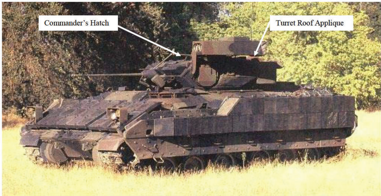
Figure 31. Titanium Commanders Hatch and Roof Applique on M2A2 Bradley Fighting Vehicle
