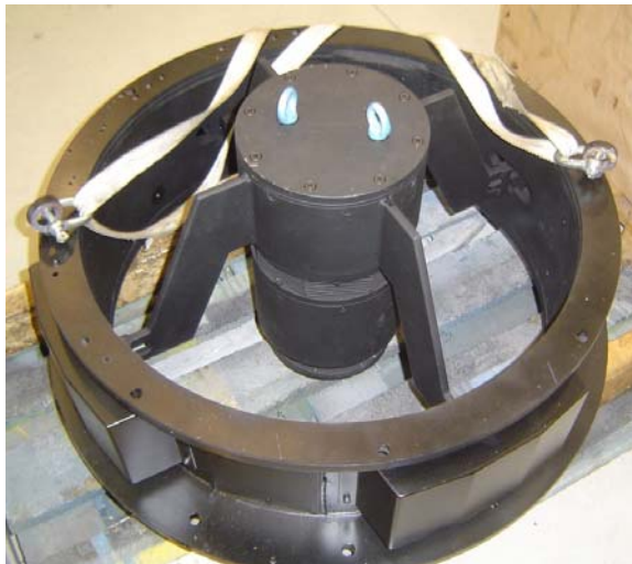
Fig.2. Spider vanes and focus support.
