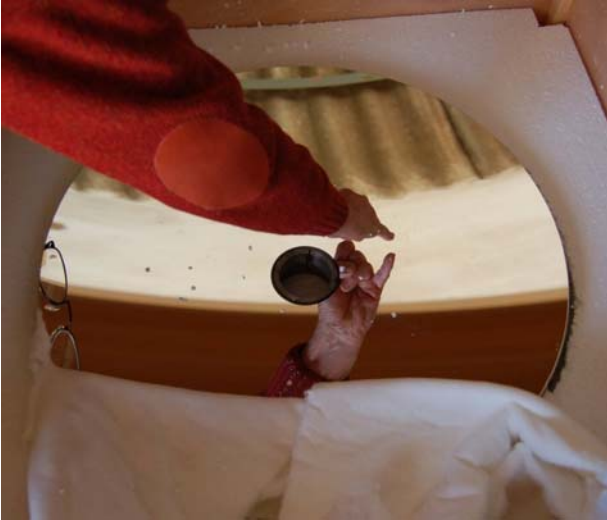
Fig.8. Realuminized mirror with SiO 2 coating.
