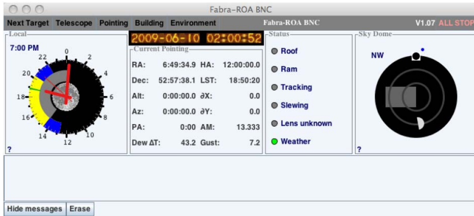
Fig.5. Main window of INDI-based control software in remote mode.
