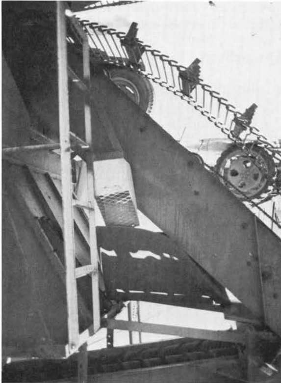
Fig. 14. Sampling can positioned on sugarbeet digger for collection of soil shaken from beet roots during harvesting. (Courtesy Herb Quick.)
