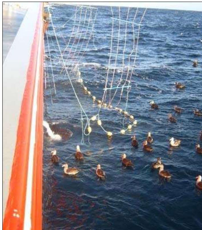
Figure 15: Photograph of a bird exclusion device (BED) of the type required for all vessels operating in CCAMLR Subarea 48.3 (note that this photograph was taken in daylight, and that night-setting of gear is required by CCAMLR and GSGSSI) [Source: CCAMLR, 2014]
