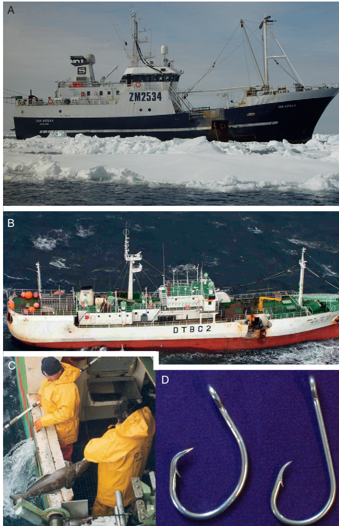
Figure 4.10 The fishery for Patagonian toothfish ( Dissostichus eleginoides ): (A) photograph of an autoliner; (B) aerial photograph of a Spanish double-line longliner, note the hauling area on the starboard side; (C) toothfish being gaffed; (D) circle-type (left) and J-type hooks used in the South Georgia fishery.
