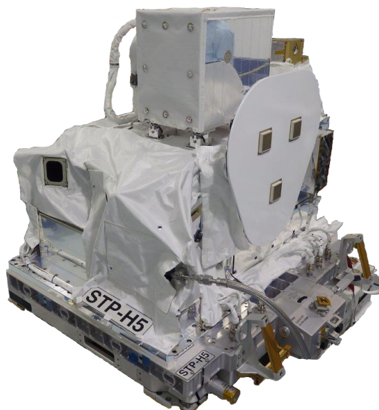
Figure 2. This image of STP-H5 shows the ground plane and three patch antennas, which face the aft direction. The FOTON GPS receiver sits under the thermal blanket toward the viewer.
