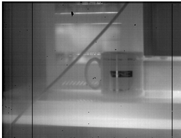
Figure 5. Two Point Temperature Corrected Image at T = 21.7 °C
