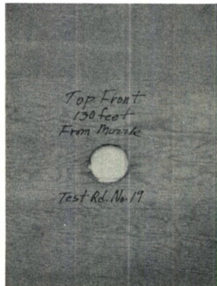
Photographs of \frac{1}{4} -inch plywood bursting screens used on the 10 June 1959 recovery shoot. Note: Fin marks as projectile passed through the plywood indicating yaw on these rounds.
