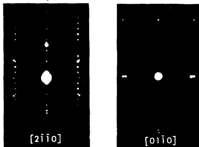
Figure 7. Selected area diffraction patterns of as-deposited Ti/SiC interface region in cross-section. Ti deposited on (0001) 6H-SiC at 400°C.
