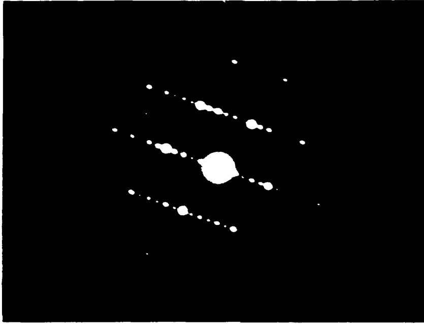
Figure 4: Selected area diffraction pattern of \beta -SiC film and 6H-SiC substrate.
