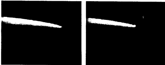
(a) Before breakdown (b) After breakdown Fig. 1 In-situ observation of both electrodes before and after the electrical breakdown.
