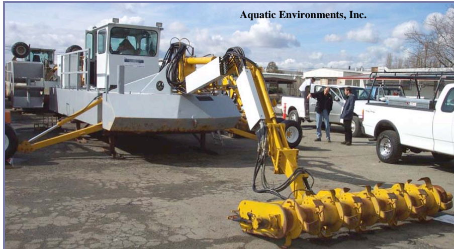
Figure 5-4. AEI "Aquamog" with rotovator arm
