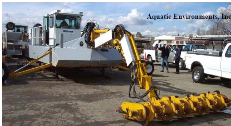
Figure A-3. "Aquamog" with Rotovator Arm
