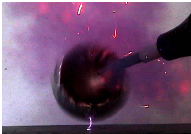
Figure 10 – Ignition of \text{I}_2\text{O}_5 On Aluminum Pan
