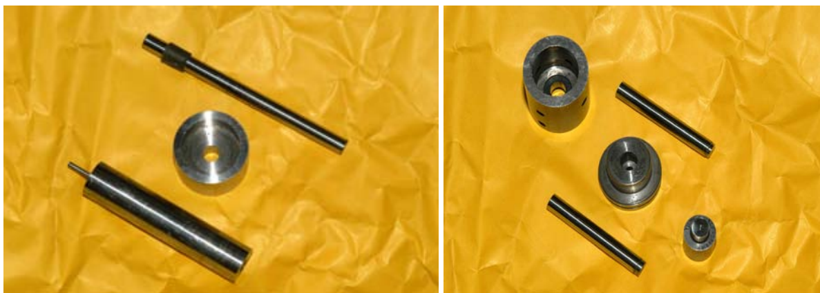
Figure 15 – Rams and Dies Used to Load MIC Electric Primers
