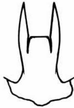
SHORT AFTBODY • AXI-SYM C-D NOZZLE WITH SPEED BUMPS
