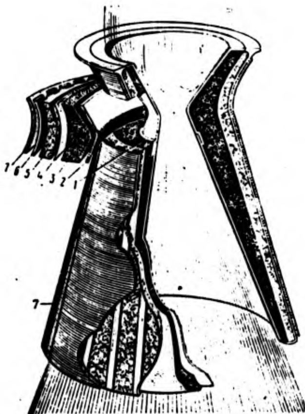
Fig. 50. Uncooled nozzle of solid-propellant rocket engine can have complex laminar construction: 1 - tungsten inner shell, flowed around by gases with a temperature of the order of 3000^{\circ}\text{C} ; 2 - intermediate layer of heat-resistant material, for example, carbide, preventing direct contact of tungsten shell with following layer - graphite (otherwise graphite will diffuse in tungsten, lowering its mechanical qualities); 3 - graphite absorber of heat, transmitted by gases to nozzle; 4 - layer of ceramic insulation protecting the following layer of insulation from high temperature; 5 - plastic insulation preventing overheating of outer shell and increasing rigidity of nozzle; 6 - supporting members of nozzle - flange with strips of highly durable alloy; 7 - external shell - winding of light and durable fiber glass.
