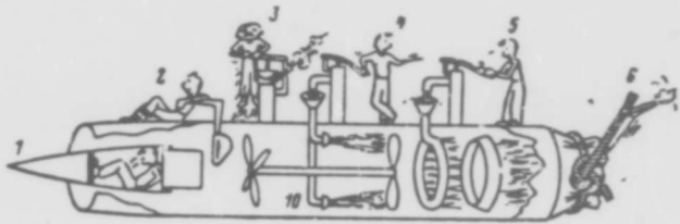
Fig. 28. A supersonic turbojet engine should have a complex automatic system for control of geometry (air inlet, compressor, nozzle), fuel feeding, and other parameters. On the figure are represented only certain necessary forms of control: 1 - adjustment of air inlet (position of central body and others); 2 - turning of compressor guide vanes; 3 - bypass of air from compressor; 4 - fuel feed in combustion chamber; 5 - fuel feed in afterburner; 6 - adjustment of jet nozzle.
