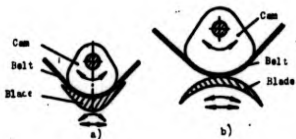
Fig. 14.7. Diagram of grinding with an abrasive belt.
