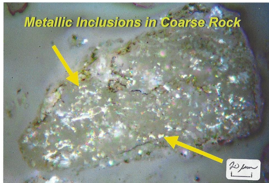
Figure 13: Photomicrographs of Koppers Samples 2020-0714 thru 2020-0720 from Geosyntec (Sediment 9- 0510, 1015 & 1520, 7-DUP-1015, 1520, 0510 & 0005) Showing; Activated Carbon in Groundmass, Fine Sized Soluble Groundmass MM, Other Coarse Rock and Metallic Inclusions. Reflected Polarized Light In Air, X600.
