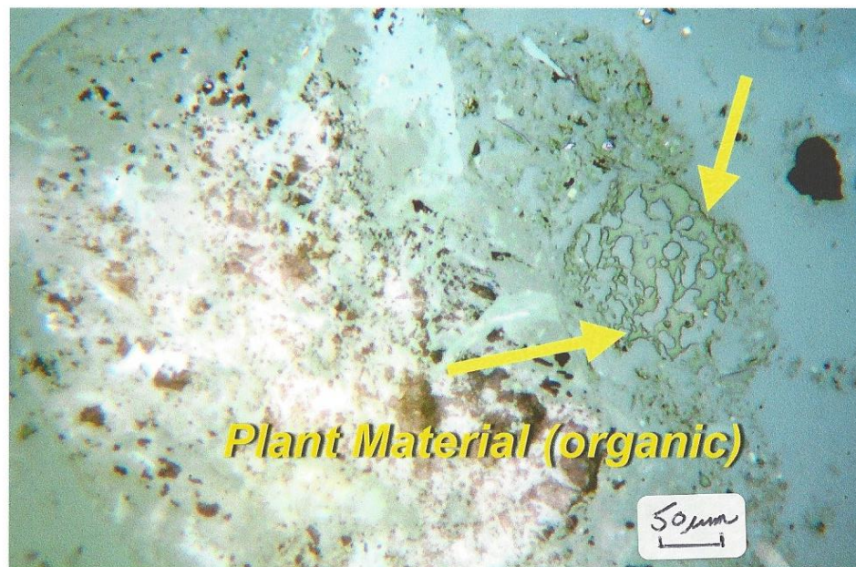
Figure 10: Photomicrographs of Koppers Samples 2020-0714 thru 2020-0720 from Geosyntec (Sediment 9- 0510, 1015 & 1520, 7-DUP-1015, 1520, 0510 & 0005) Showing; Seashell, Fine Sized Groundmass Material Coating Coarse Seashell, Activated Carbon and Plant Material (organic). Reflected Polarized Light In Air, X250.
