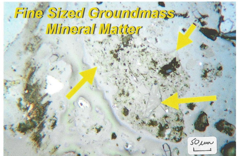
Figure 9: Photomicrographs of Koppers Samples 2020-0708 thru 2020-0713 from Geosyntec (Sediment 6-1520, 0510 & 0005, 7-1520, 0005 & 0510) Showing; Activated Carbon Mixed with Groundmass MM, Metallic Inclusions in Rock Type, Iron Oxide and Fine Grain Groundmass MM. Reflected Light In Air, X250.
