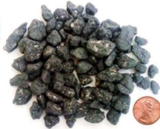
Figure 1. Configuration of PAC-coated particle.
