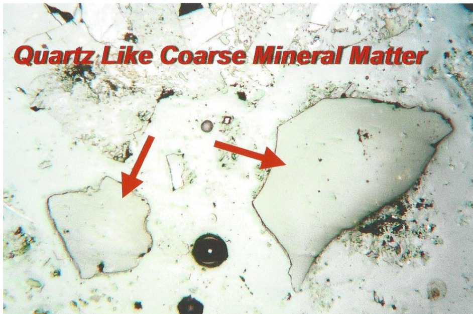
Figure 9.) Photomicrographs of Koppers Samples 2020-0695 thru 2020-0700 from Geosyntec (Sediment 2-1520, 0005 & 1015, 3-0510,1520 & 1015) Showing; Seashell – Coarse Carbonate, Activated Carbon, Quartz Like Coarse MM and Activated Carbon with Groundmass MM. Reflected Polarized Light In Air, X135.
