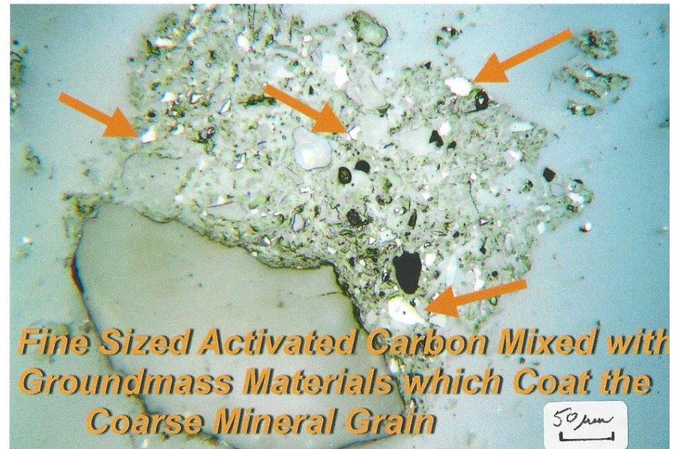
Figure 10: Photomicrographs of Koppers Sample 2020-0081 thru 20-0086 of Sediment Samples from Geosyntec (T82-2, 3, 5, 6, 7 & 9) Showing; Coal Based Activated Carbon, Groundmass Mineral Matter, Water Soluble Mineral and Fine Sized Activated Carbon in Groundmass. Reflected Light In Air, X250.
