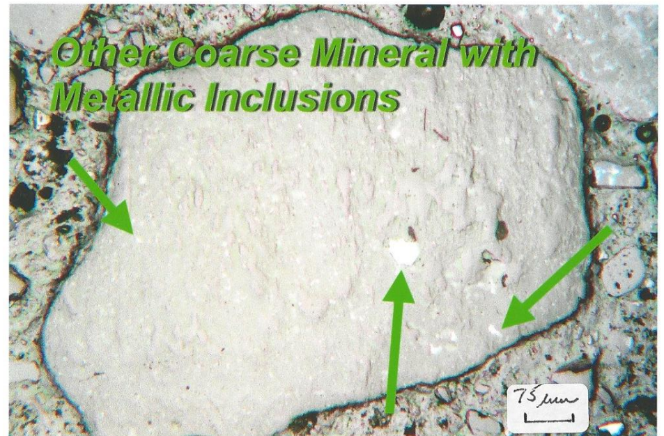
Figure 7: Photomicrographs of Koppers Sample 2020-0081 thru 20-0086 of Sediment Samples from Geosyntec (T82-2, 3, 5, 6, 7 & 9) Showing; Carbonate (dolomite/limestone), Seashell - carbonate, Quartz/Clear Mineral (sand) and Other Coarse Mineral with Metallic Inclusions. Reflected Light In Air, X135.
