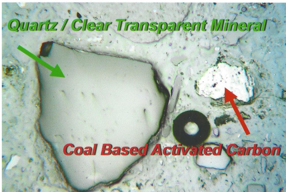
Figure 9: Photomicrographs of Koppers Sample 2020-0081 thru 20-0086 of Sediment Samples from Geosyntec (T82-2, 3, 5, 6, 7 & 9) Showing; Carbonate (dolomite/limestone), Seashell - carbonate, Quartz/Clear Mineral (sand) and Other Coarse Mineral with Metallic Inclusions. Reflected Light In Air, X250.
