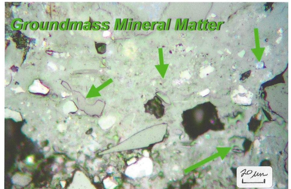
Figure 12.) Photomicrographs of Koppers Samples 2020-0695 thru 2020-0700 from Geosyntec (Sediment 2-1520, 0005 & 1015, 3-0510, 1520 & 1015) Showing; Seashell - carbonate, Activated Carbon with Groundmass MM, Coarse Carbonate (limestone) and Groundmass Mineral Matter. Reflected Polarized Light In Air, X600.
