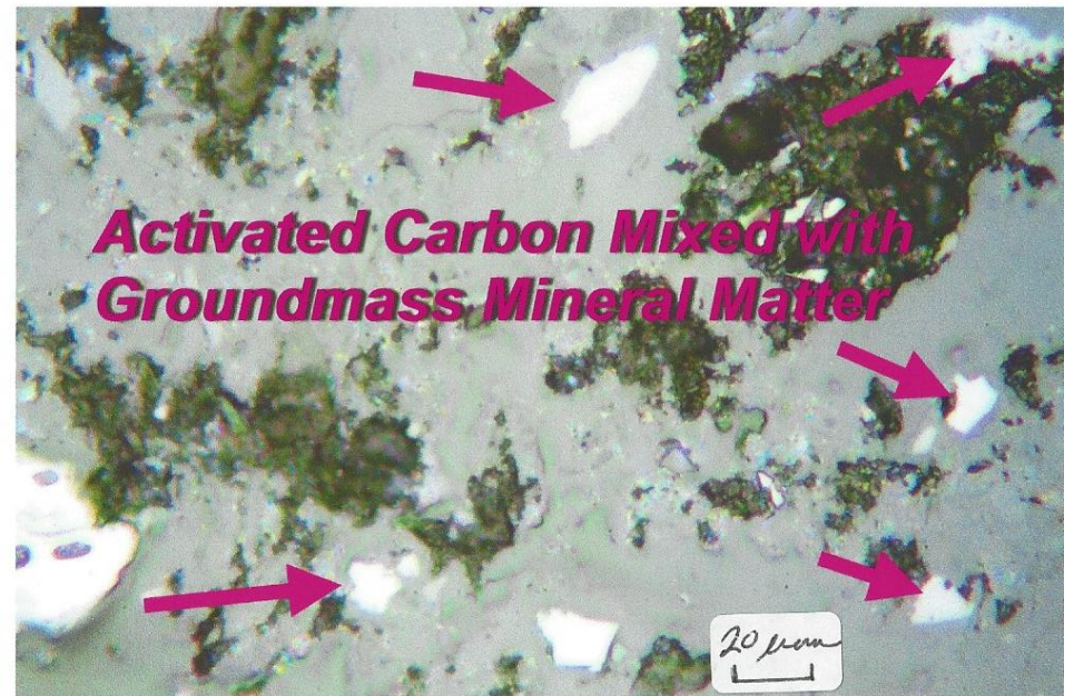
Figure 13: Photomicrographs of Koppers Samples 2020-0701 thru 2020-0707 from Geosyntec (Sediment 4-1520, 0510, 0005 & 1015, 5-0510, 1520 & 1015) Showing; Calcite, Other Coarse MM, Partially Soluble MM, Pyrite Aggregate and Activated Carbon Mixed with Groundmass Mineral Matter. Reflected Light In Air, X600.
