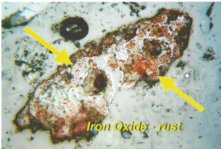
Figure 9: Photomicrographs of Koppers Samples 2020-0708 thru 2020-0713 from Geosyntec (Sediment 6-1520, 0510 & 0005, 7-1520, 0005 & 0510) Showing; Activated Carbon Mixed with Groundmass MM, Metallic Inclusions in Rock Type, Iron Oxide and Fine Grain Groundmass MM. Reflected Light In Air, X250.
