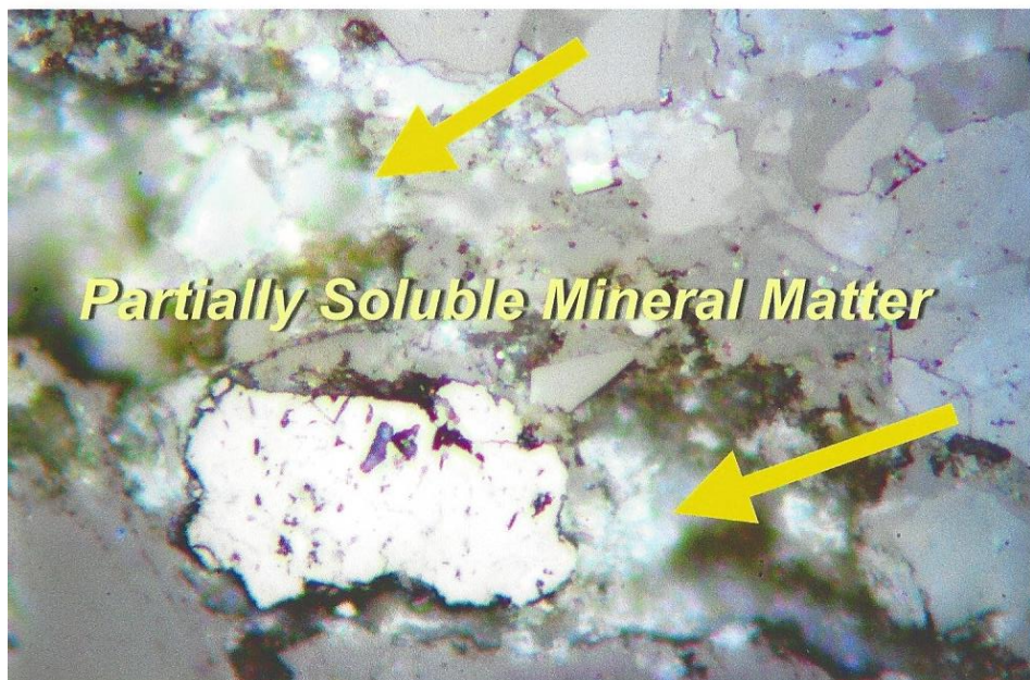
Figure 11: Photomicrographs of Koppers Samples 2020-0708 thru 2020-0713 from Geosyntec (Sediment 6-1520, 0510 & 0005, 7-1520, 0005 & 0510) Showing; Quartz-like Mineral, Activated Carbon Mixed with Groundmass MM, Partially Soluble MM and Metallic Inclusions in Coarse MM. Reflected Light In Air, X600.
