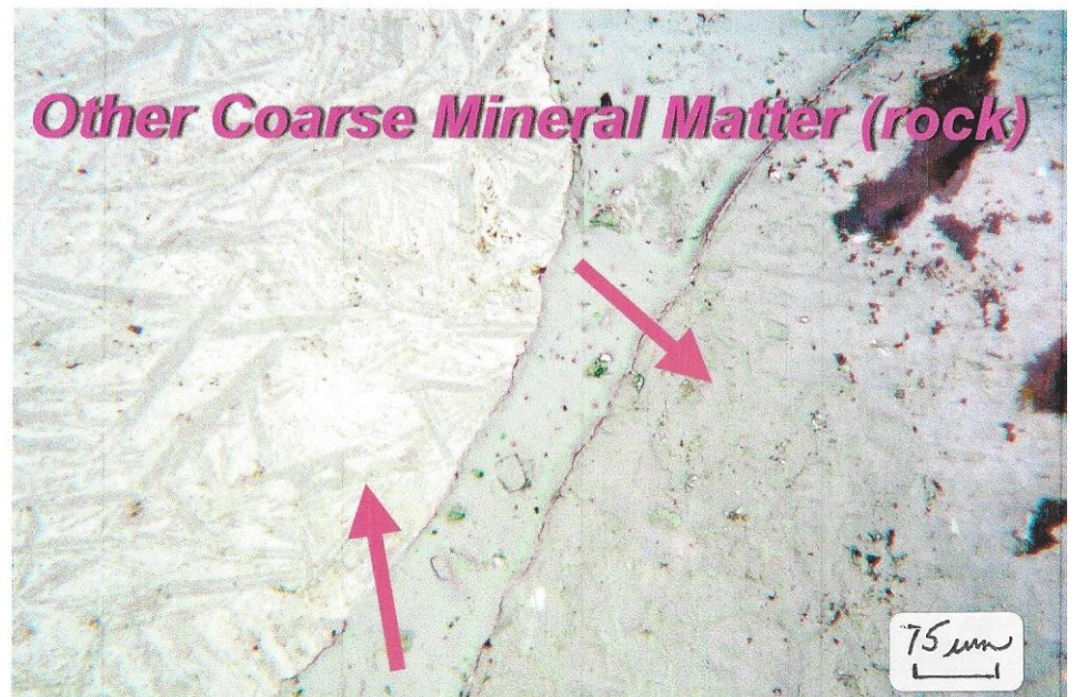
Figure 7: Photomicrographs of Koppers Samples 2020-0695 thru 2020-0700 from Geosyntec (Sediment 2-1520, 0005 & 1015, 3-0510,1520 & 1015) Showing; Sea Shell (carbonate), Coarse Carbonate (limestone), Quartz Like Coarse Mineral Matter and Other Coarse Mineral Matter (rock). Reflected Polarized Light In Air, X135.
