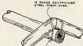
18 GAUGE GALVANIZED STEEL STRAP WRAPPED AROUND BOTH RAFTERS AND UNDER RIDGE BEAM, ATTACHED WITH 50MM CLOUTS
