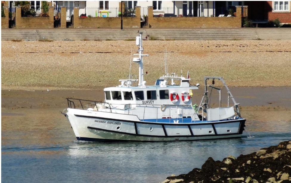
Figure 5: Wessex Explorer – Survey vessel used to undertake baseline benthic grab and DDV surveys
