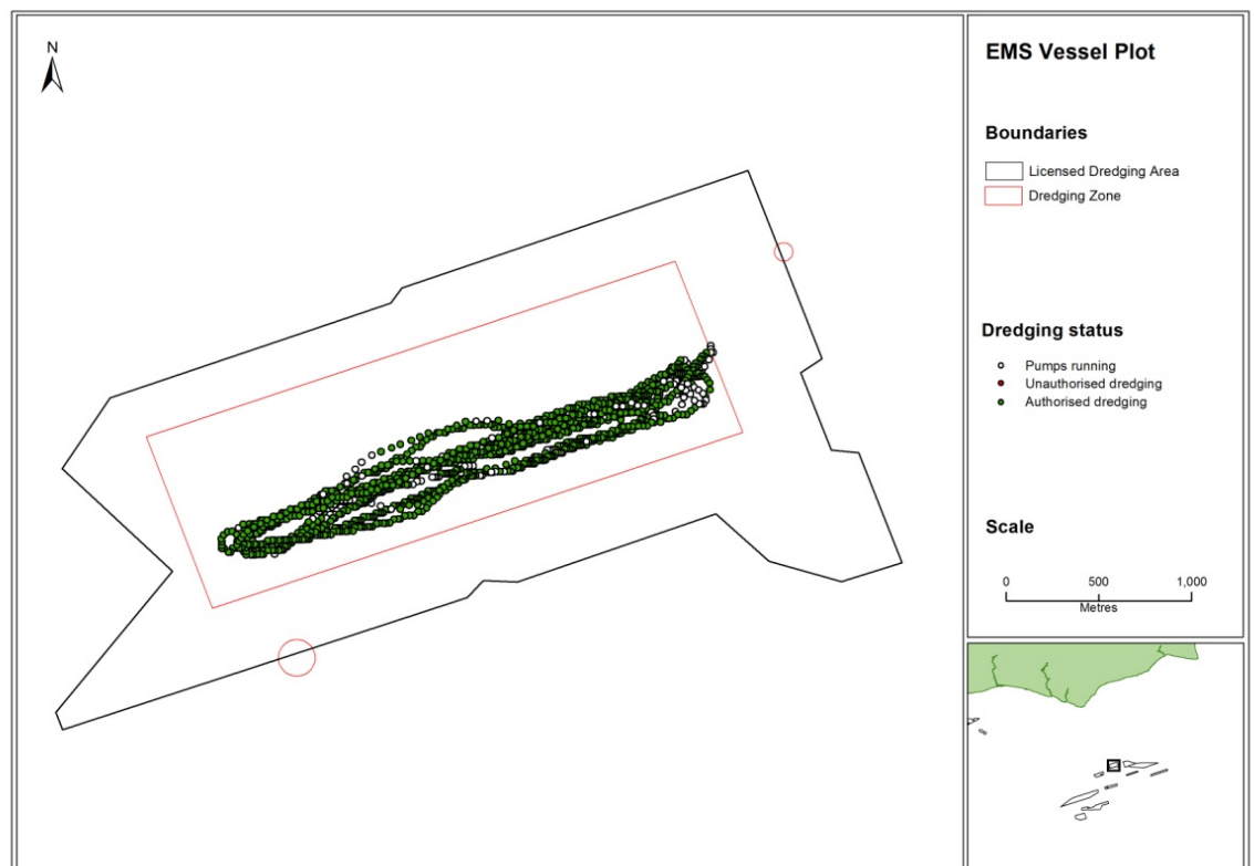
Figure 2.7. An example of a track plot derived from the UK electronic monitoring system. The position and status of the vessel (pump on/dredging) is recorded every 30 seconds while dredging is taking place, using a combination of GPS and sensors associated with the dredge gear.
