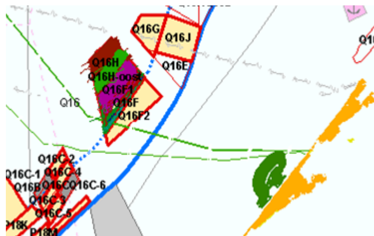
Figure 2.5. An example of the Dutch monitoring and registering system (MARS), which shows track plots of different hopper dredgers within licence areas during extraction for the Sand Motor project (21.5 million m 3 ).
