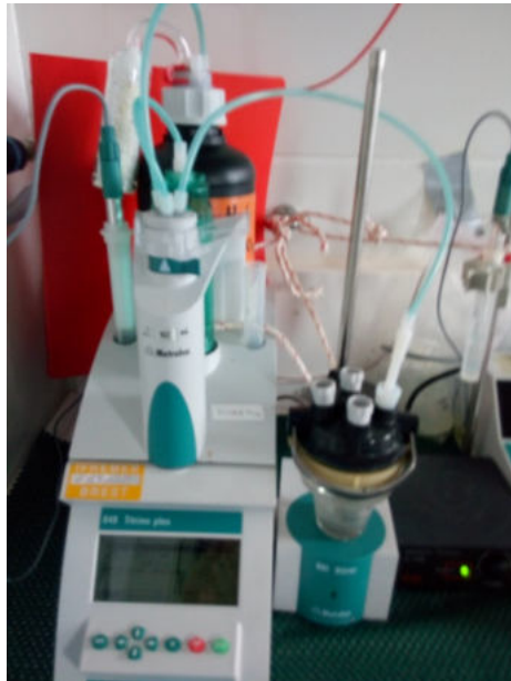
Figure 11: Metrohm Titrino used for the [H 2 S] measurement. © Ifremer – Chubarc 2019 Cruise.
