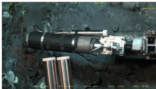
Figure 9: example of hot fluid sampling with BEG gastight bottle. © Ifremer – Chubarc 2019 Cruise.
