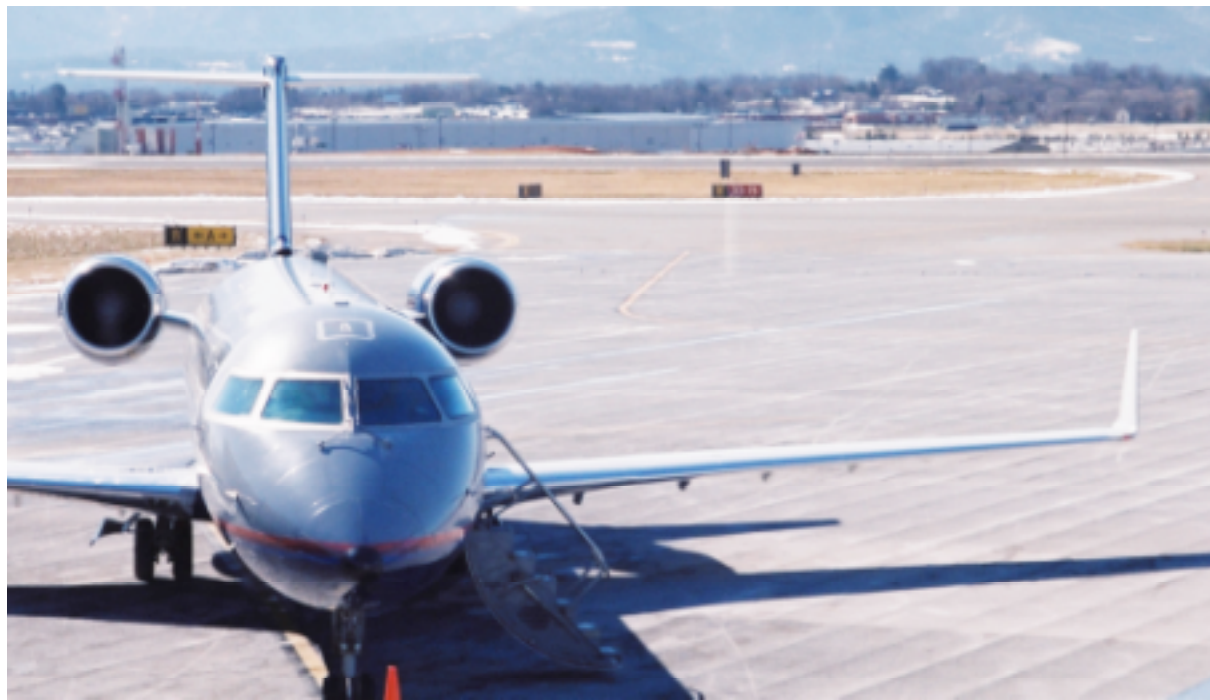
Figure 4-8. Winglet on a Canadair Regional Jet at Roanoke, Virginia Airport, January 2003
