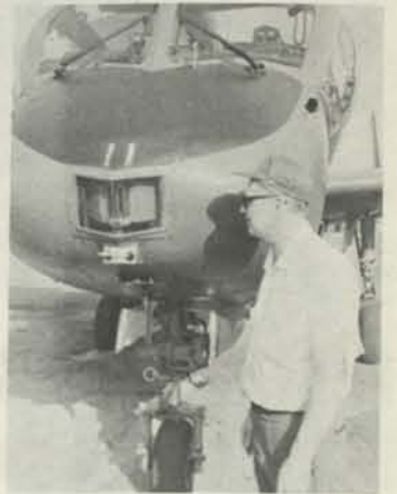
LOU KEVITZ looks over the forward oblique installation of the Fairchild KA-60B panoramic camera in the U. S. Army Mohawk aircraft. Lou just returned from a seven-month tour of duty for Fairchild in Vietnam.
