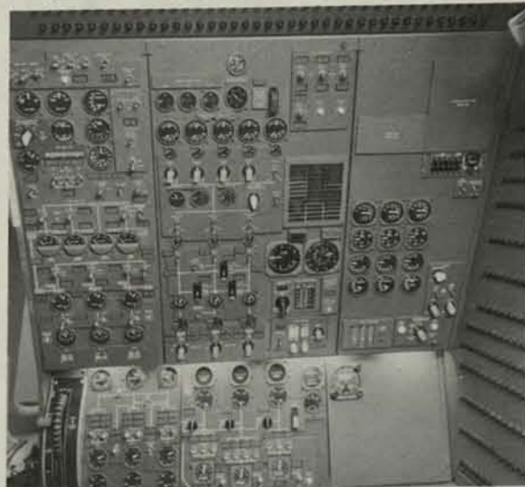
At the Flight Engineer's station, the Fairchild Flight Data Recorder occupies the upper right portion of the control panel.
