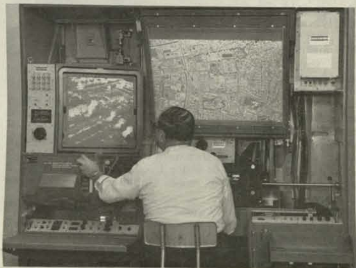
A FAIRCHILD TECHNICIAN checks out the Imagery Interpretation Station prior to shipment. Designed, developed and manufactured by Fairchild Space and Defense Systems, the IIS presents a variety of photographic records in direct, magnified, or screen-projected displays in support of the Photo Interpreter.
