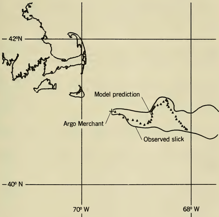
Figure 2-12. Predicted and observed location and shape of oil slick, December 22. Model prediction shows oil released from the Argo Merchant from 1000, December 17, through 1000, December 22. Wind input is from Nantucket Light Ship.
