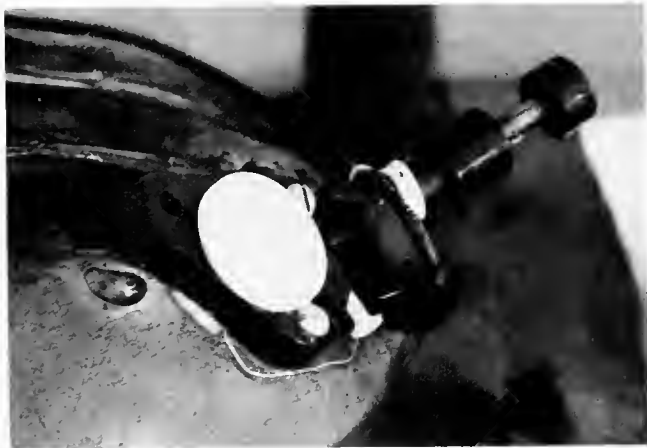
Figure 1. Chamber for recording optic nerve activity in situ from Limulus underwater. The lateral optic nerve exits the eye on the left, travels under the carapace and runs through the chamber on the right on its way to the brain. The microsuction electrode is shown inserted into the chamber from the right.
