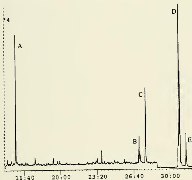
Fig. 2. Chromatogram of the derivatized (with BSTFA) reaction of *Triepolus distinctus* glandular pouches. Peak "A" = unidentified, two active hydrogen groups, two oxygens, and a molecular weight of 259. Peak "B" =  $C_{16}$  fatty acid. Peak "C" = a long-chain fatty acid TMS ester. Peak "D" = monounsaturated  $C_{18}$  fatty acid TMS ester. Peak "E" = a saturated stearic acid TMS ester. Peaks "A," "B," and "C" are magnified times four.
