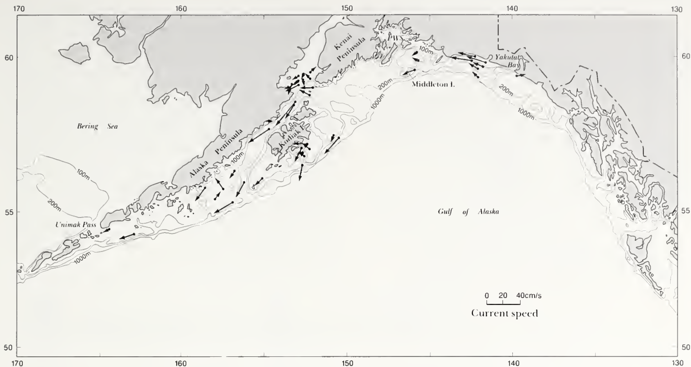
Figure 3-14. Approximate net current speeds and directions derived from the current data in Table 3-2.
