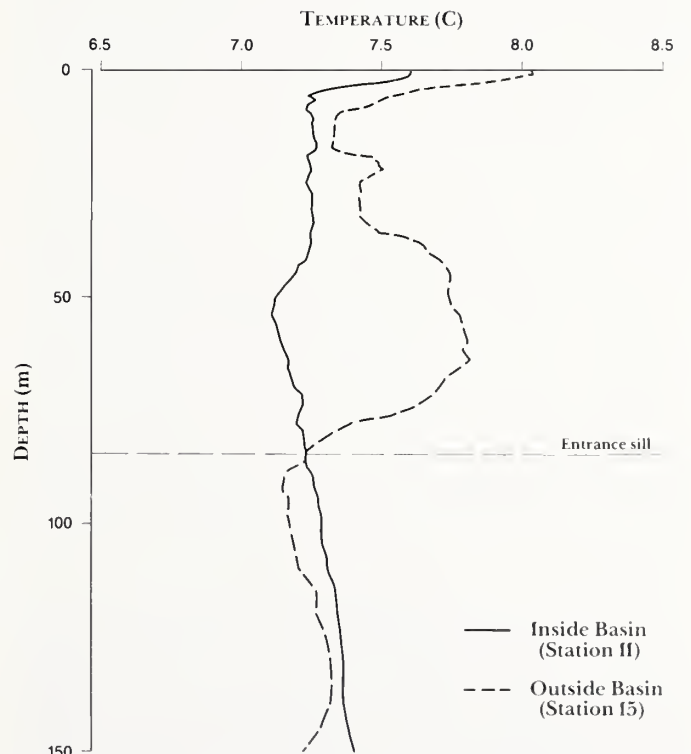
Figure 7-7. Vertical temperature profiles outside and inside the entrance sill of Boca de Quadra fjord, April 1983. (See Fig. 7-27 for longitudinal profile.)
