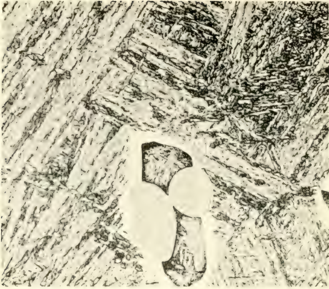
1. Freda meteorite: Kamacite with inclusions of phosphide eutectic. Picral etching. × 500.
