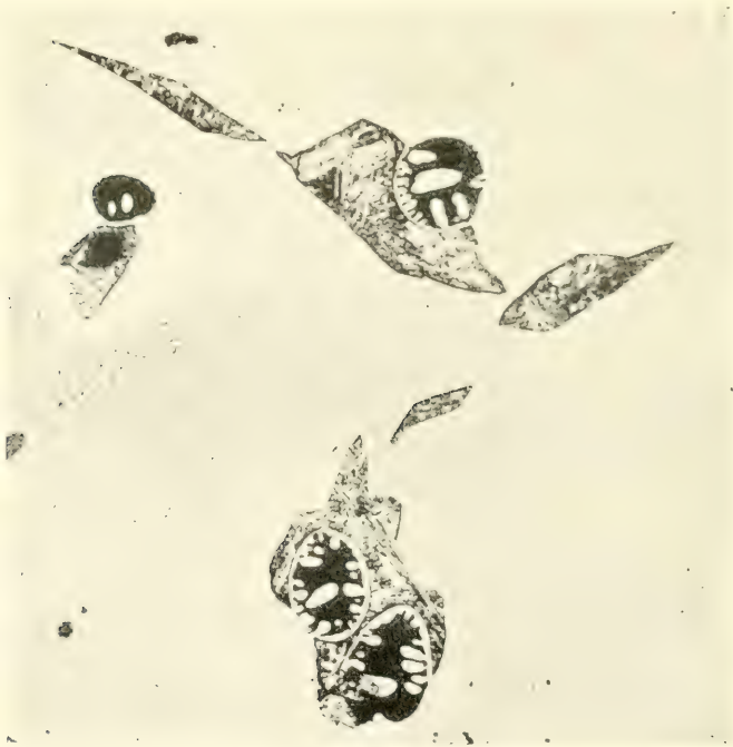
2. Eutectic inclusions. Sodium picrate darkens the phosphide inclusions. Clear areas are rejected iron droplets. × 250.
