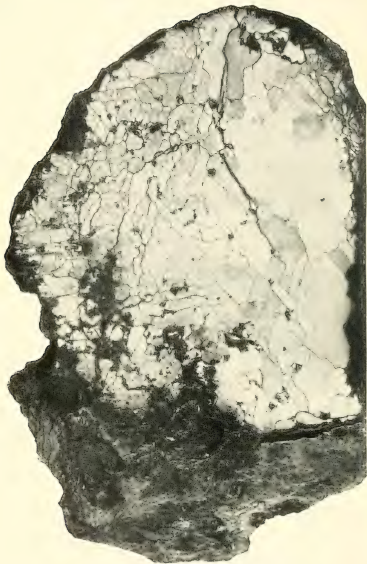
Coarse octahedrite (natural size). This section was cut from a fragment found by the authors. The dark weathered zone at the left slopes down from the plane of the polished face.
