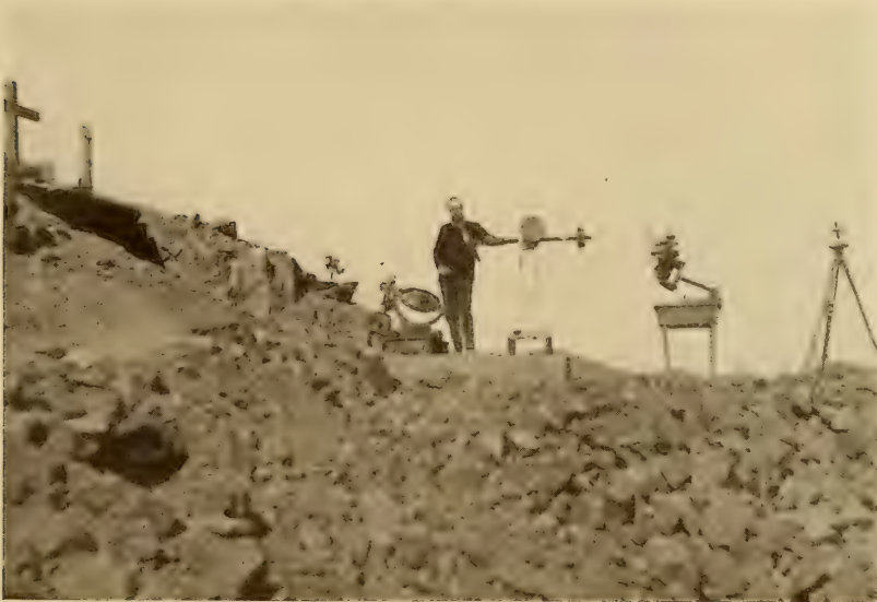
FIG. 33.—Pyranometer, coelostat, pyrhelimeters and theodolite with L. H. Abbot, Director at Mount Montezuma.
