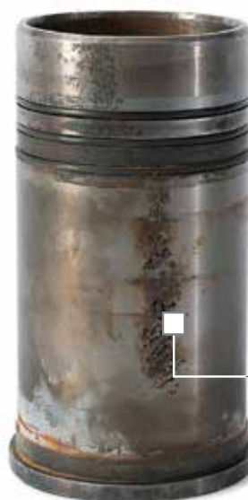
Imploding bubbles damage liners...
