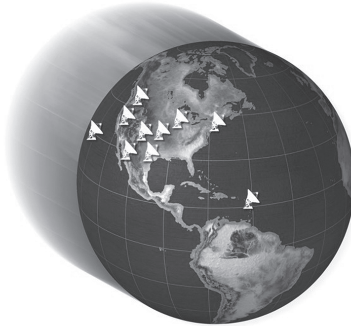
Figure 1.5. The Very Long Baseline Array (VLBA) of 10 25-m telescopes extending 8000 km from St. Croix, VI to Mauna Kea, HI yields angular resolution as fine as \theta = 0.00017 arcsec, surpassing the resolution of the Hubble Space Telescope by two orders of magnitude. Image credit: NRAO/AUI/NSF.
