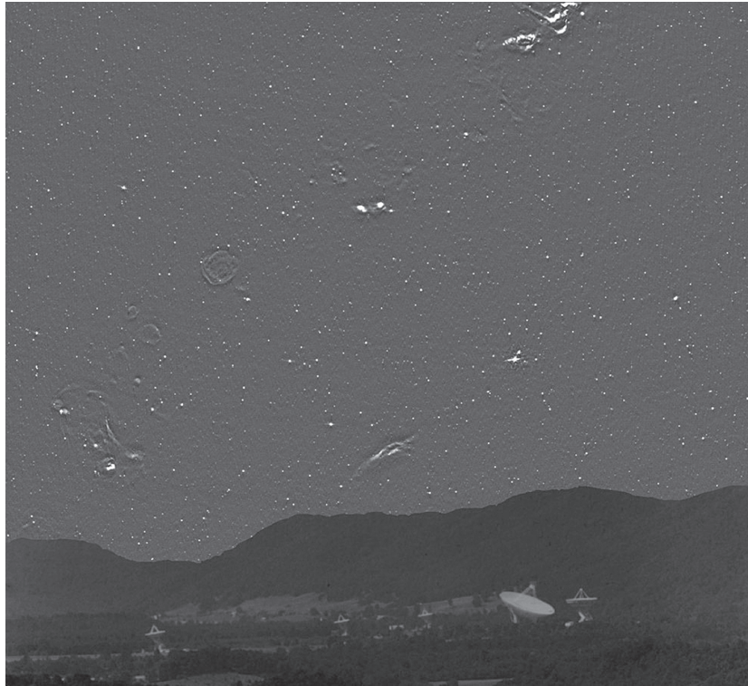
Figure 1.9. The radio sky is shown above an old photograph of the NRAO site in Green Bank, WV. The former 300-foot telescope (the largest dish) made this 4.85 GHz radio image [27], which is about 45 degrees across. Increasing radio brightness is indicated by lighter shades to indicate how the sky would appear to someone with a “radio eye” 300 feet (91 m) in diameter. Image credit: NRAO/AUI/NSF. Investigators: J. J. Condon, J. J. Broderick, and G. A. Seielstad.
