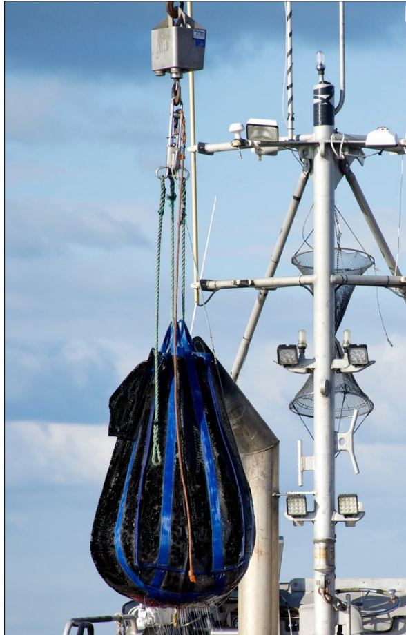
Figure 2-6. Example of a brailer to transfer plastic onto the plastic extraction vessel.
