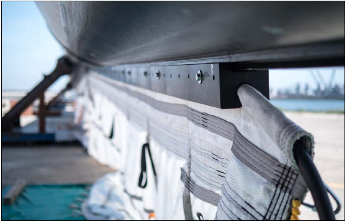
Figure 2-2. Screen clamping bracket used to connect the screen to the Ocean Cleanup System.
