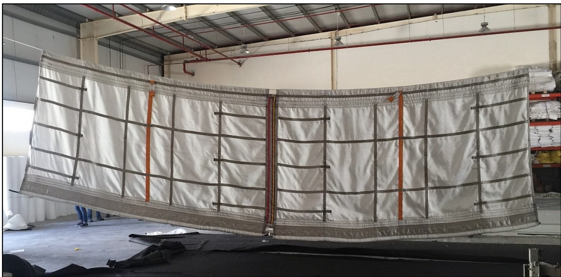
Figure 2-3. Small section of the impermeable screen that is part of the Ocean Cleanup System.
