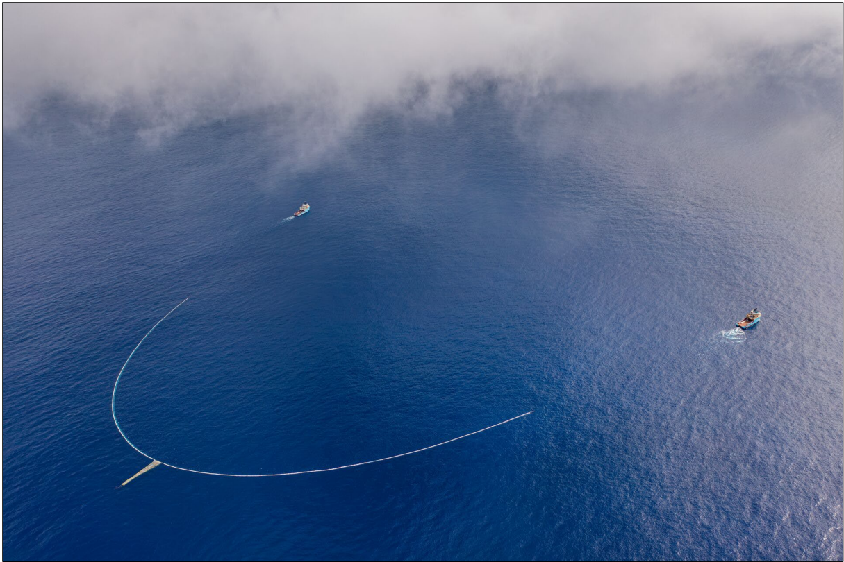
Image ES-1. S03 towing lines (connected to each ship), Retention System (white wings and submerged net), and retention zone (blue and yellow net attached to the back of the Retention System).
