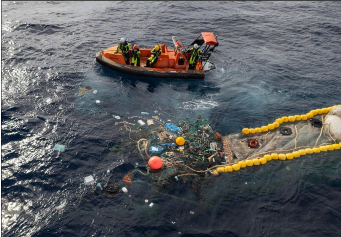
Image 2-6. Plastics released from the retention zone after activation of the electric release.
