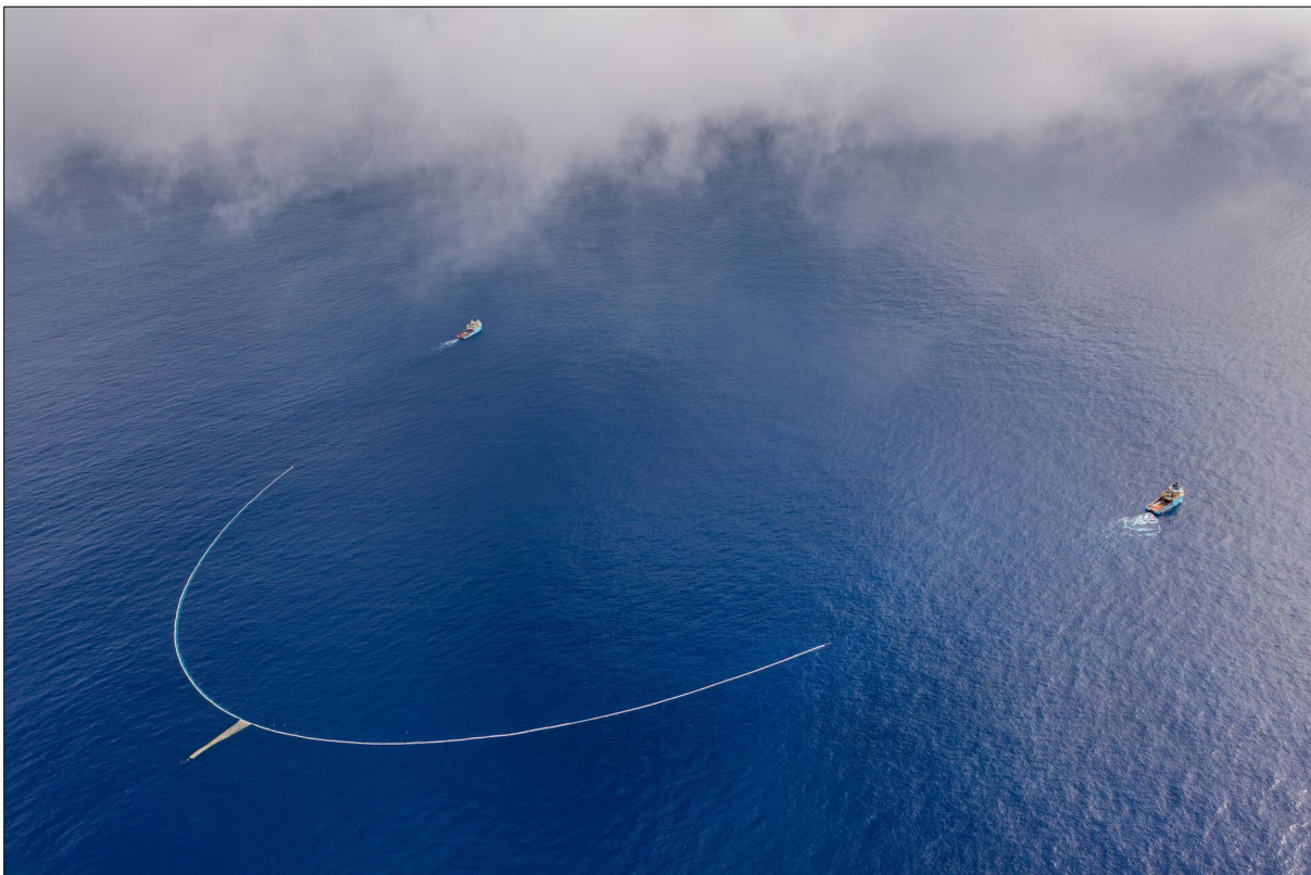
Image 2-8. S03 towing lines (connected to each ship), wings with submerged net, and retention zone.
