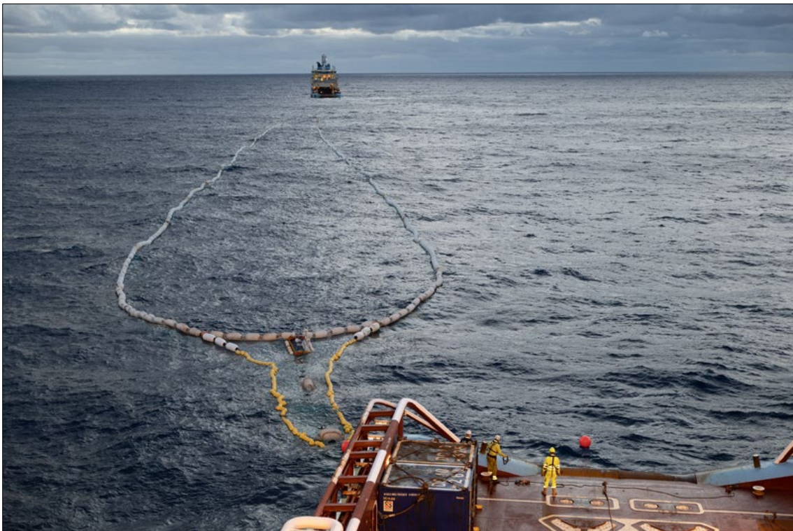
Image 9. Shortened retention zone being towed by one vessel during plastics extraction operations.
