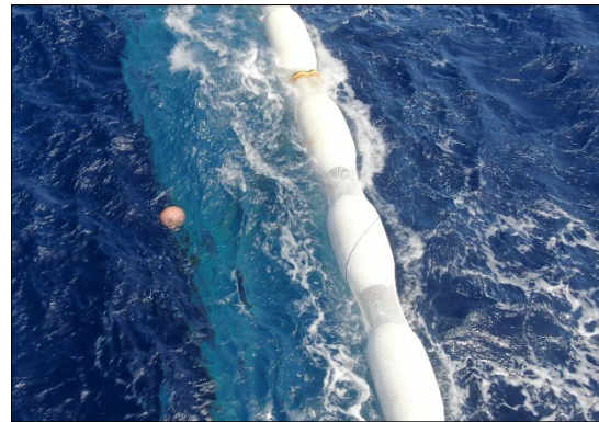
Image 4-1. Overtopping of the S002 wings.
