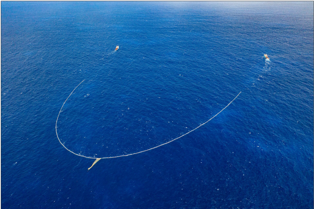
Image 2-1. S002 Retention System towing lines (connected to each ship), wings with submerged net), and retention zone (net attached to the back of the Retention System) (Image Credit: Toby Harriman).
