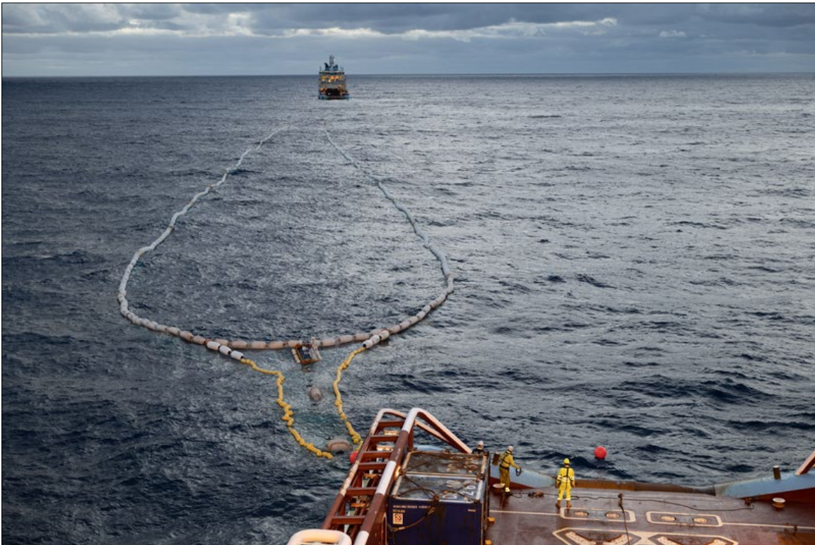
Image 2-11. Shortened retention zone being towed by one vessel during plastics extraction operations.
