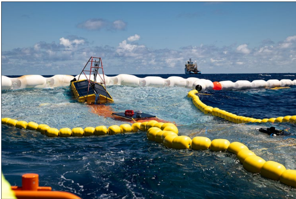
Image 4. Camera skiff unit mounted on top of the retention zone entrance.
