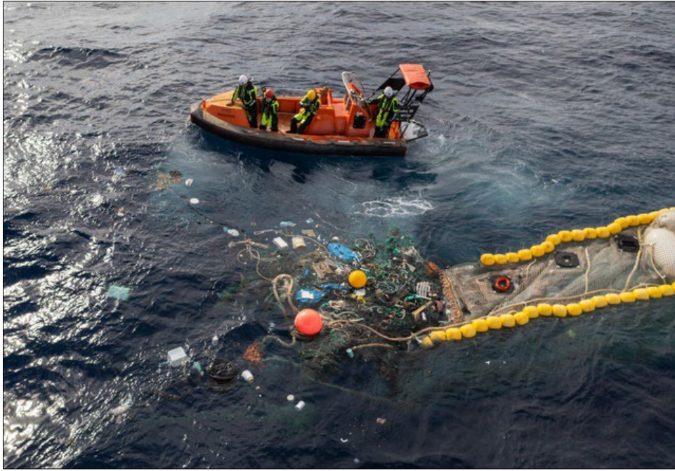
Image 6. Plastics released from the retention zone after activation of the acoustic release.
