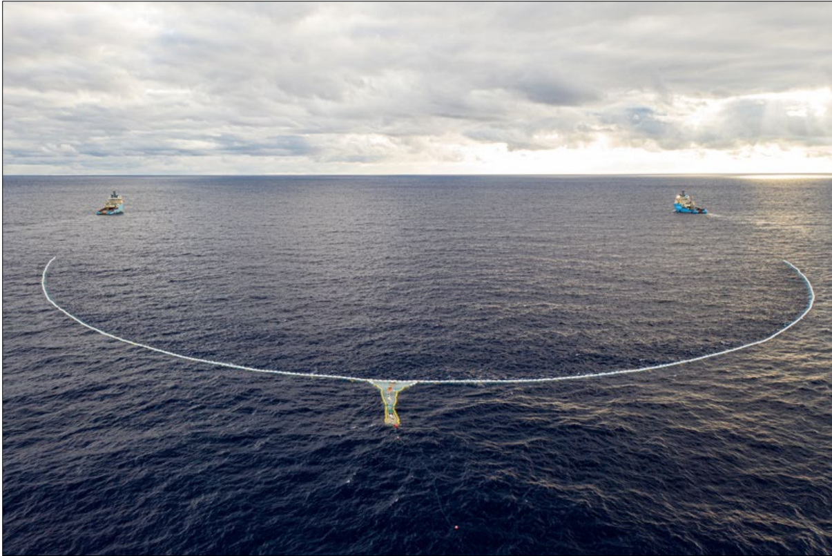
Image 1. Towing lines (connected to each ship), retention system (white wings and submerged net), and retention zone (blue and yellow net attached to the back of the retention system).
