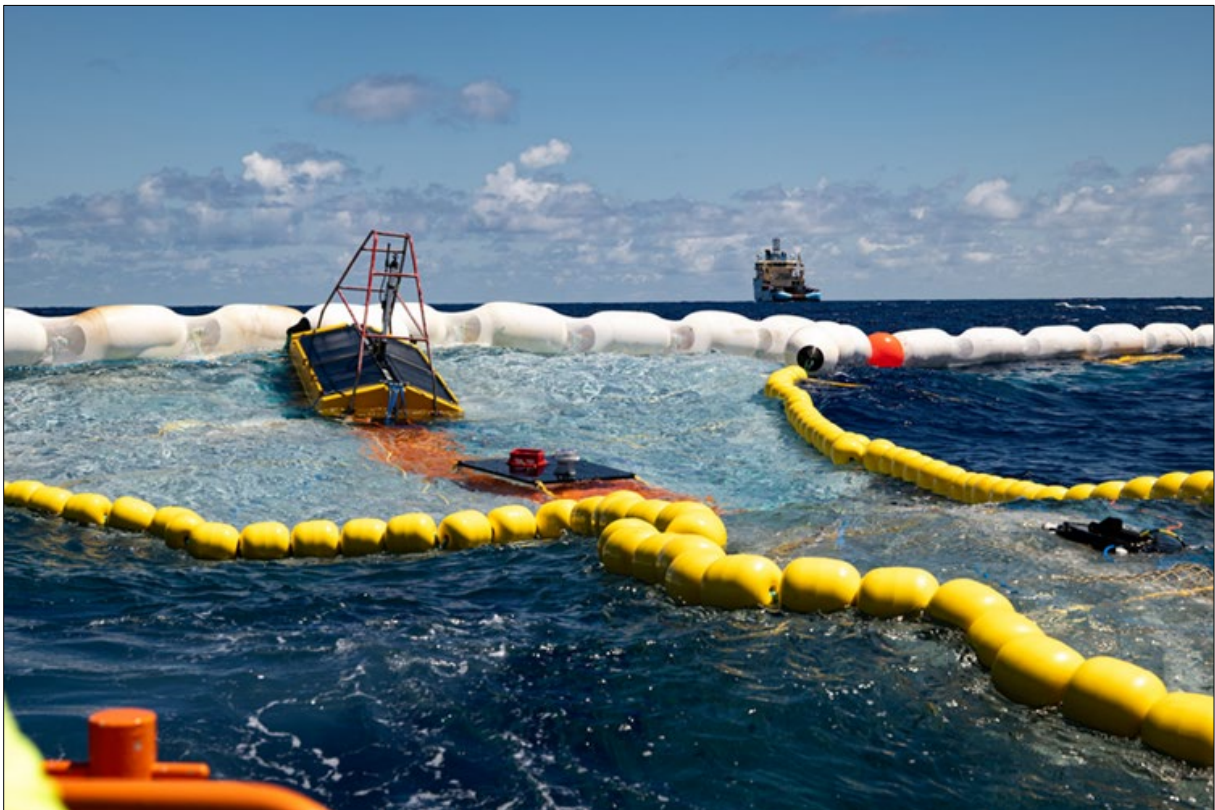
Image 2-4. Camera skiff unit mounted on top of the S002 retention zone entrance.
