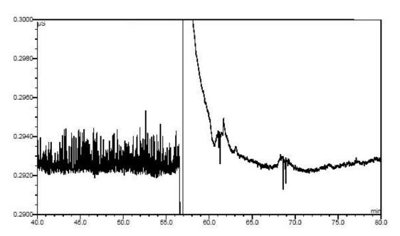
**Figure 29** Effect of Air Bubbles on Baseline Dionex ADRS 600 (4 mm), Recycle Eluent Mode
