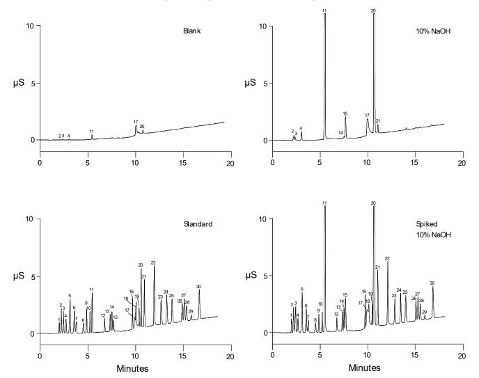
Table 24 Recovery Data for the Dionex IonPac AS11 Analysis of 10% NaOH
