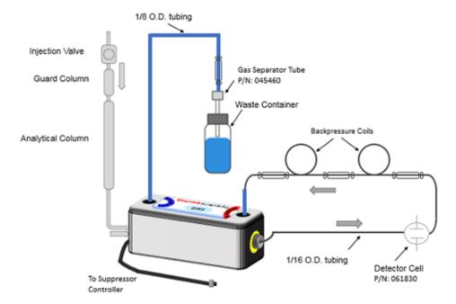
Figure 5 System with back coils
