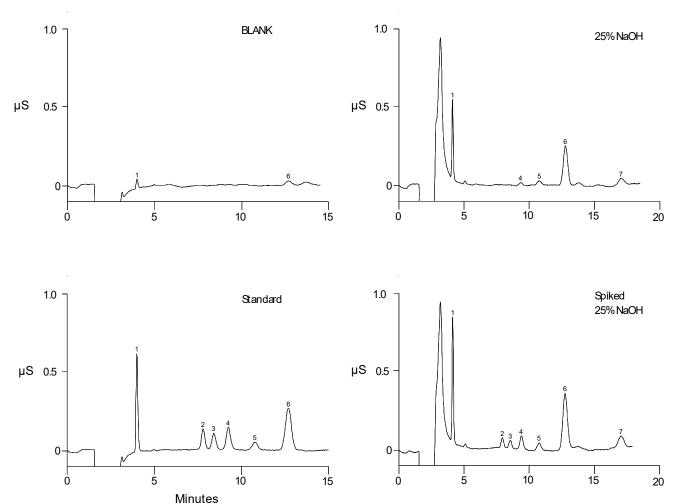
**Figure 21** Dionex IonPac AS12A Isocratic Analysis of Blank, Standard, 25% NaOH Sample and Spiked 25% NaOH Sample
