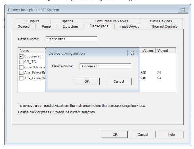
Figure 12 Suppressor configuration in Integrion
