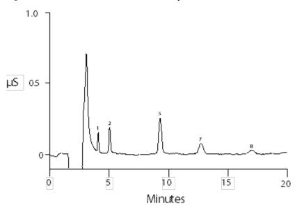
Figure 22 Dionex IonPac AS12A Analysis of 20% Ammonium Hydroxide
