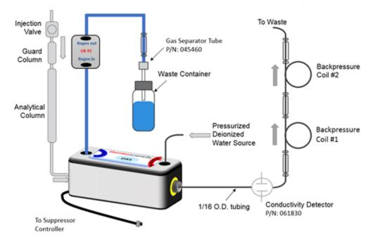
Figure 16 AutoSuppression External Water Mode plumbing diagram
