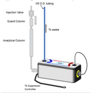
Turn on the pump and flow ≤10 mM eluent or DI water at **0.5 mL/min** for 4mm suppressor or **0.125 mL/min** for 2mm suppressor for 20 minutes. **The power to the suppressor must be turned off during this step.**
