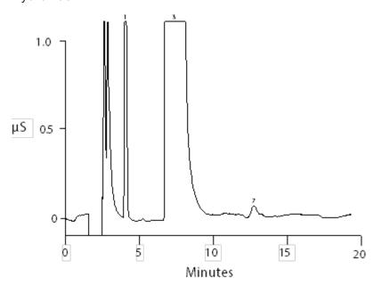
**Figure 23** Dionex IonPac AS12A Analysis of 25% Tetrabutylammonium Hydroxide
