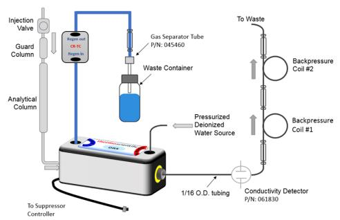
Any analysis that can be performed using the AutoSuppression Recycle Mode can be done using the AutoSuppression External Water Mode. A constant source of deionized water having a specific resistance of 18.2 megohm or greater is supplied to the regenerant chambers to generate hydronium or hydroxide ions for suppression.
