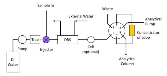
Figure 19 The Dionex DRS 600 Neutralization Mode Plumbing Diagram
