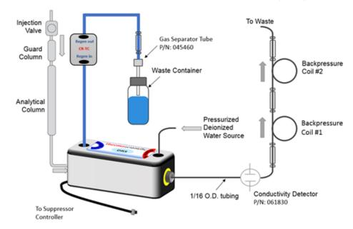
Figure 17 AutoSuppression External Water Mode Plumbing Diagram
