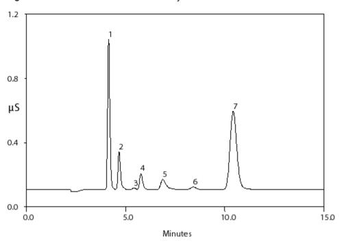
Figure 26 Dionex IonPac CS12A Analysis of 25% Acetic Acid
