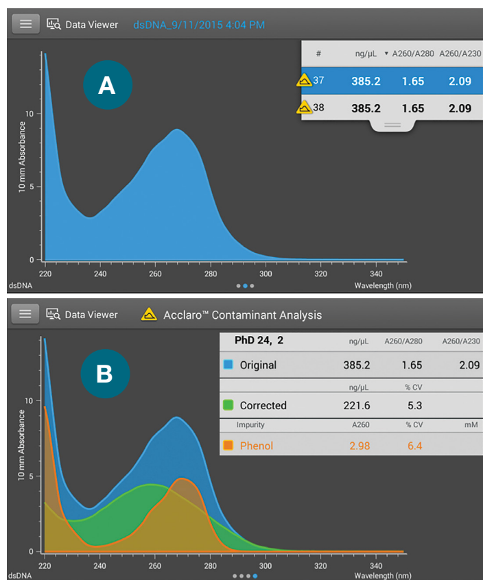
Figure 1: The Acclaro Contaminant ID feature identifies possible contaminants present in a sample. 1A) Measurement screen: the Acclaro Contaminant ID icon indicates that the Acclaro algorithms have detected a potential contaminant in a dsDNA sample. 1B) Contaminant analysis screen: comparison of original absorbance spectrum (DNA plus phenol, blue), the corrected spectrum (original minus contaminant, green) and the contaminant spectrum (orange). This screen also contains the original and corrected DNA concentration results.
