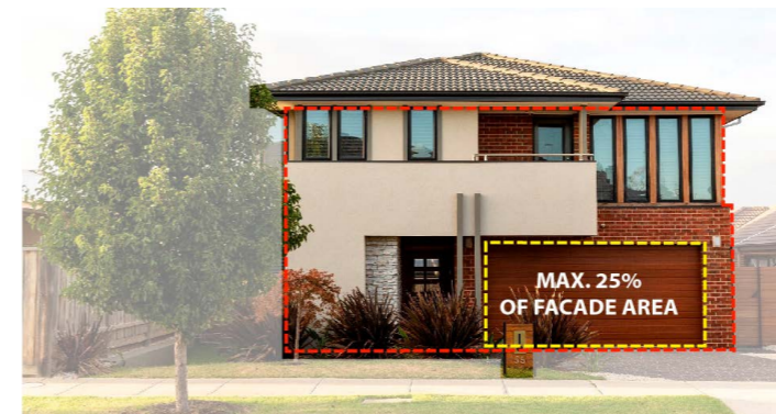
Figure 24: For a house with upper levels, the area of the garage opening must be no more than 25% of the area of the front facade.
