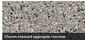
Chosen exposed aggregate concrete
