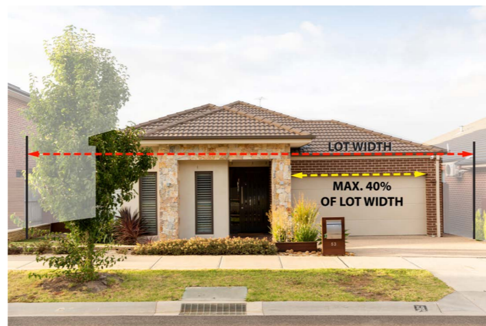
Figure 23: The garage opening(s) for a single storey house must be no wider than 40% of the lot width.
