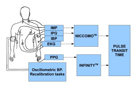
Figure 2.7: Pulse Transit Time Diagram
