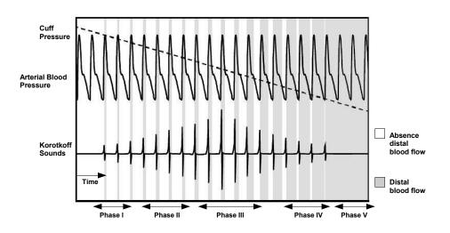
Figure 2.5: Fundamentals of Auscultatory Method
