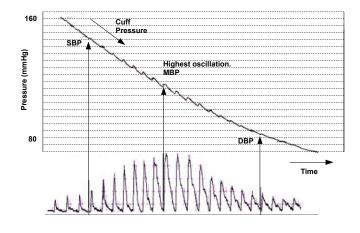
Figure 2.6: Oscillometric Method
