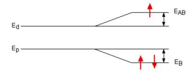
**Fig.11** Energy levels  $E_d$  and  $E_p$  for the *d* and *p* orbitals,  $E_{AB}$  and  $E_B$  for the antibonmoding and bonding molecular orbitals.
