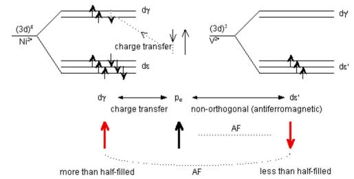
**Fig.38** Schematic representation of the superexchange interaction (Ni<sup>2+</sup> -  $p_{\sigma}$  – V<sup>2+</sup>) in the 90° case.
