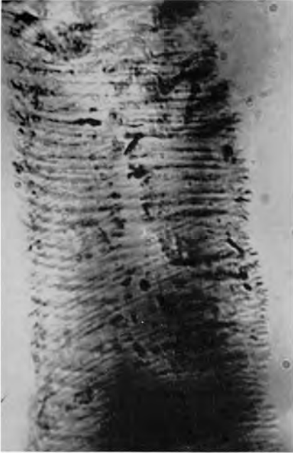
Fig. 17 — Fibrillar patterns of the tertiary wall of spruce There are two sets of threads — one with transversal orientation ( 87^\circ ), another with an inclination of 65^\circ (see discussion, page 31)
