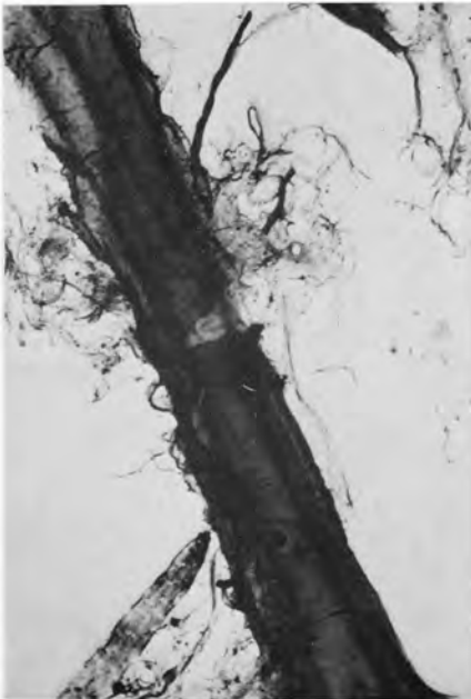
Fig. 6 — Beaten spruce fibre The primary wall is separated: dark lines of incrustated zones are built into the secondary wall and lie under the primary wall
