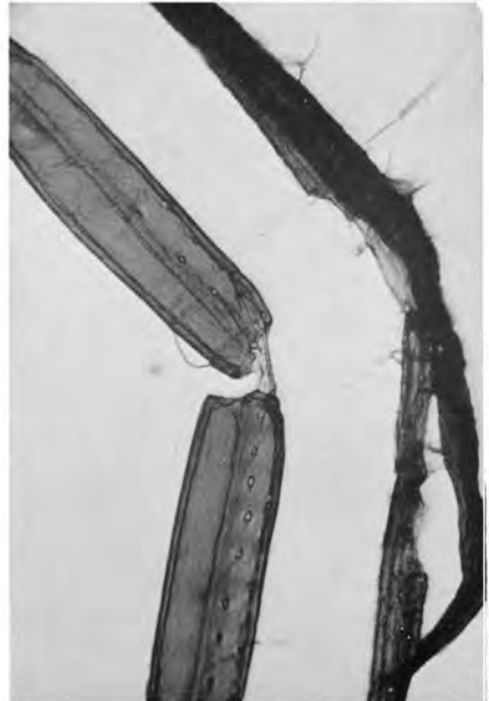
Fig. 7 — Spruce fibre cut by beating action The broken pieces are connected with the more resistant pit zone of the wall
