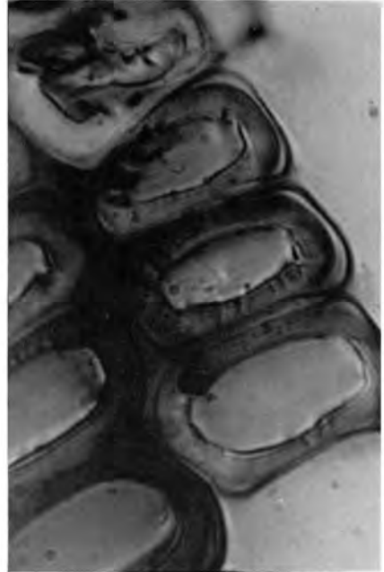
Fig. 8a — During maceration of wood, an exterior layer of the cell (primary wall?) has become separated from the fibre
