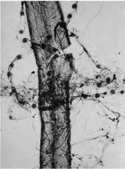
Fig. 8b — An exterior layer is separated when beating a fibre: it is suggested that it is the primary wall, as the closing membranes (tori) of the pits are connected with this layer
