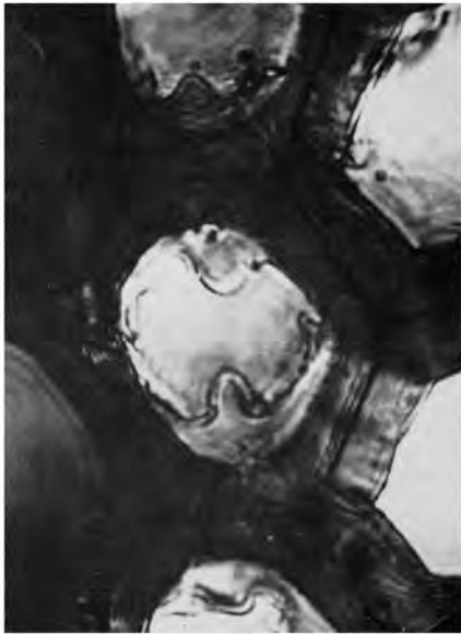
Fig. 9 — When macerating wood sections, a lamella came off the fibre inside the secondary wall (spruce)
