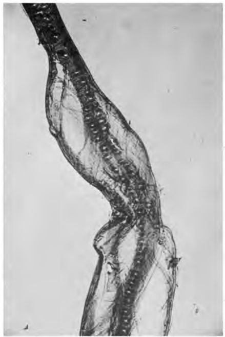
Fig. 3 — Pit zone resists deformation when crushing the fibre
