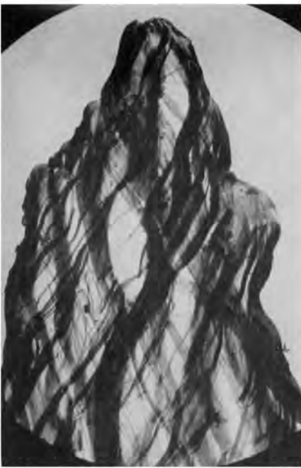
Fig. 1 — Tip of a spruce fibre, crushed The separated fibril bundles represent a 'microscopic continuity': the fibrillar strands do not terminate at the tip, they are looped in steps
