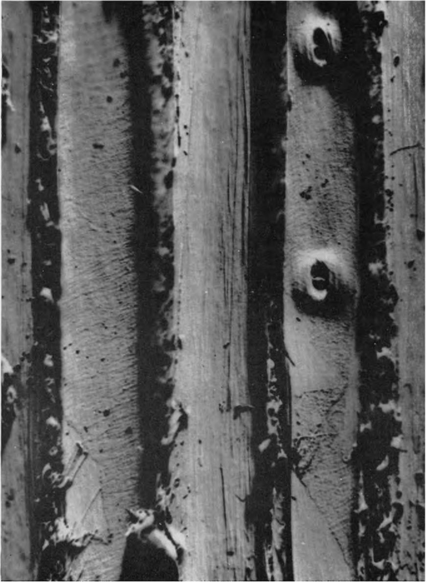
Fig. C — A radial surface of Norway spruce — the cut has passed through the lumina (light micrograph \times 1020 )
