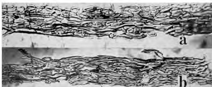
Fig. 6—Section through handsheets made from (a) late wood fibres and (b) early wood fibres from Pinus taeda
