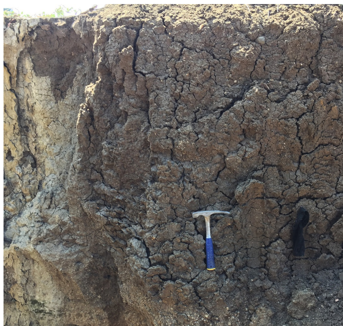
Fig. 7 Deep clay-lined cracks (plan view to left and cross sections to right) produced by vertization in a Vertisol, near Savner, Maharashtra, India. Geology hammer for scale is 25 cm long.
