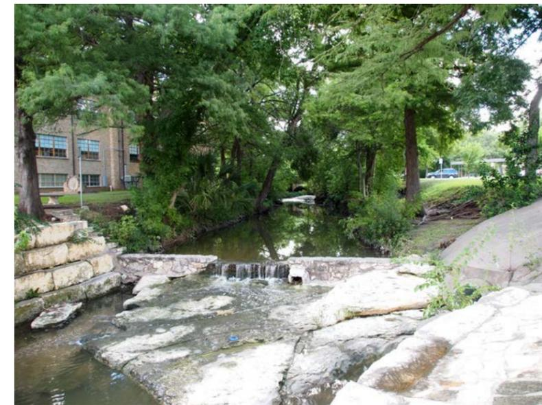
In stream structures should be removed to reduce the elevation of water profiles and avoid reverse hydraulic supercritical flows of floodwaters below the structures.
