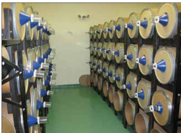
Figure 2. Cardboard rearing barrels, with funnels and vials inserted into the lids, into which emerald ash borer adults collect following their emergence from logs inside barrels. This is an efficient system for rearing adult beetles from field-harvested beetle-infested logs. (Photo credit: Jonathan Lelito, USDA APHIS PPQ)
