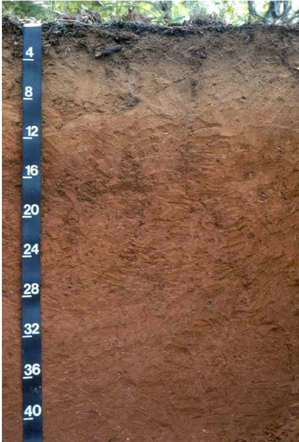
Profile of a Paleudult in Alabama. The ochric epipedon consists of a darkened surface layer and an underlying grayish brown layer that extends to a depth of about 10 inches. This epipedon is underlain by a thick, red argillic horizon that extends beyond the base of the photo. Scale is in inches.
