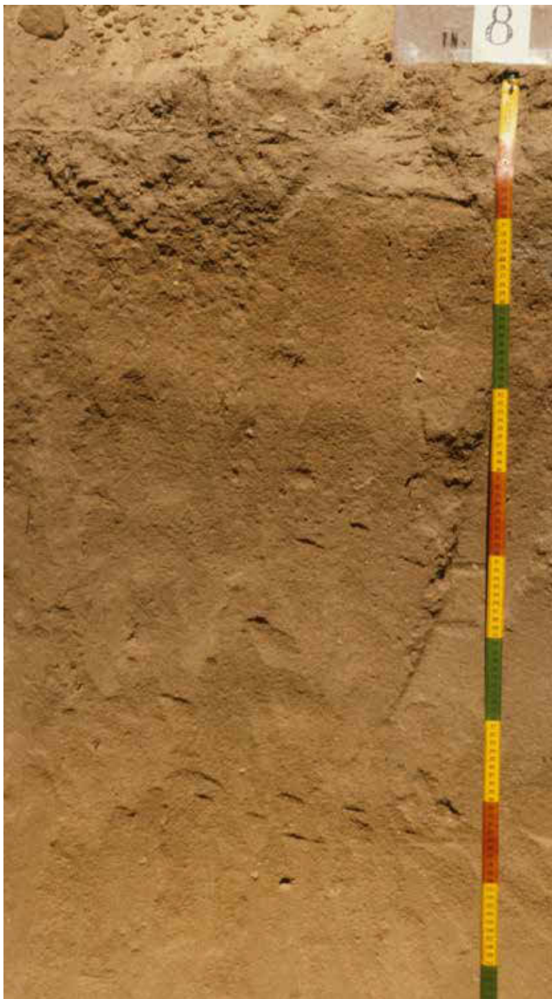
Profile of a Xerept (specifically a Haploxerept) in Tunisia. This soil has a reddish brown cambic horizon between depths of about 10 and 60 cm. Scale is in cm.
