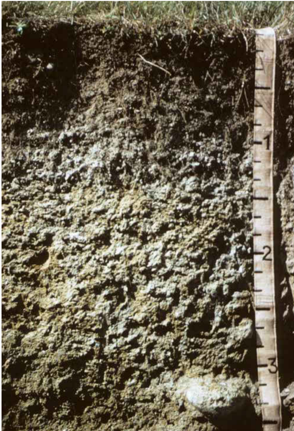
Profile of an Aquept (specifically a Humaquept) in Maine. The soil has an umbric epipedon extending to a depth of about 13 inches and a gray cambic horizon with redoximorphic features extending to depths below the base of the photo. Scale is in feet.
