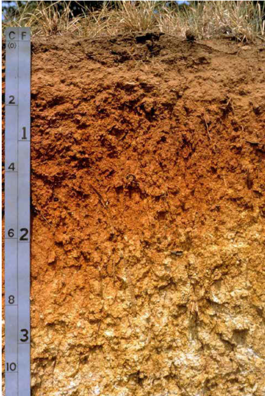
Profile of a moderately well drained, clayey Haplustult in Texas. This soil has an ochric epipedon consisting of a darkened surface layer (about 7 cm thick) and an underlying lighter-colored layer from which clay has been leached (between depths of 7 and 18 cm). Below this epipedon is a yellowish red argillic horizon that becomes reddish yellow to gray in the lower part.
