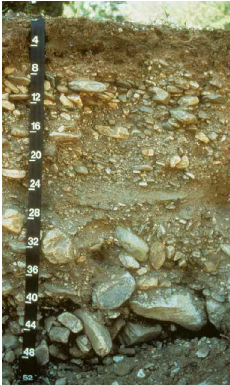
Profile of an Orthent (specifically a Udorthent). This soil formed in gravelly, cobbly, and stony colluvium. Other than the ochric epipedon, it has no other diagnostic horizons. Scale is in inches.
