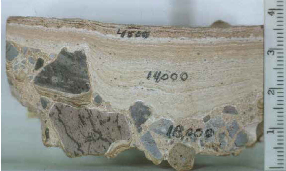
Cross-section of the upper part of a petrocalcic horizon with a laminar cap. The penciled numbers are the ages of various parts of the layer. Scale is in inches.
