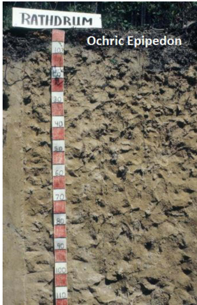
Profile of an Andisol with a thin ochric epipedon that has been darkened by organic matter. Scale is in cm.
