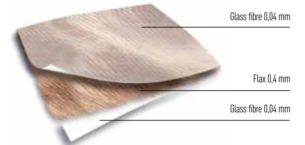
FLAX® sandwich cone 6 1/2" (165 mm) woofer cone conception
