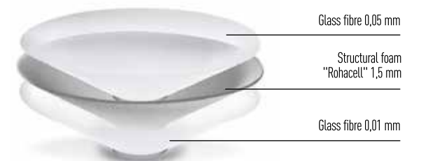
"W" Sandwich cone 6 1/2" (165 mm) woofer cone conception
