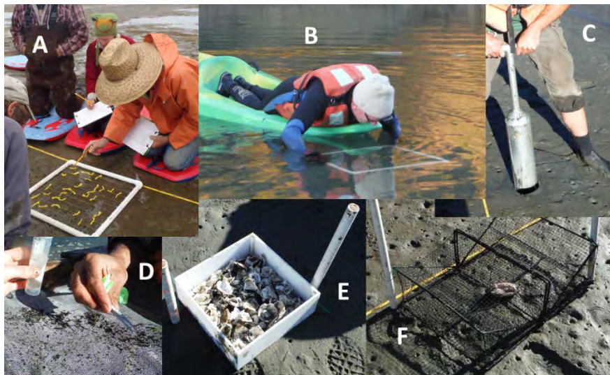
ES 1. Sampling methods for macrophytes and invertebrates, including training (A), using a kayak for quadrat sampling in order to minimize disturbance (B), sampling infauna with the clam gun (C), sorting infauna on the sieving screen (D), box trap with oyster shell (E), and crab trap (F).
