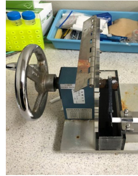
B) Using Plant Microtome MTH-1 for cross section branch root into 20 µm thickness
